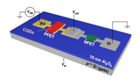
By depositing gold (Au) and Indium (In) contacts, researchers create two crucial types of quantum dot transistors on the same substrate, opening the door to a host of innovative electronics. Credit: Los Alamos National Laboratory
